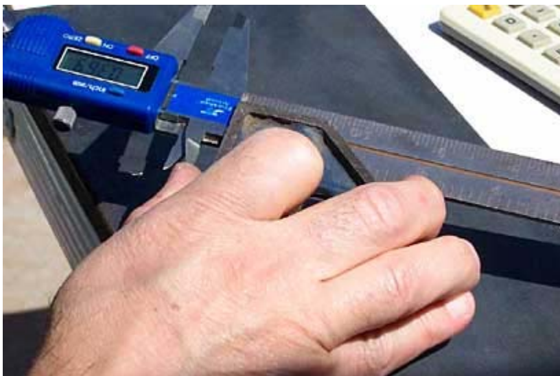
Using the caliper to set the sliding square for scribing the horizontal inboard holes.
