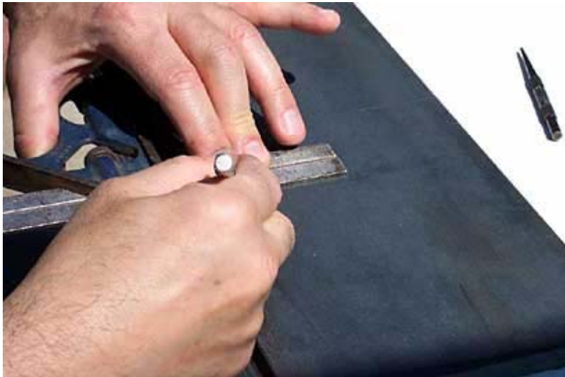
Scribing the line for the vertical or Y-axis center-to-center measurement of right inboard hole.
