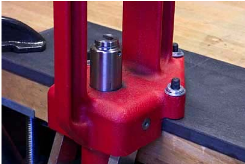
Flat washers & lock washers installed.
