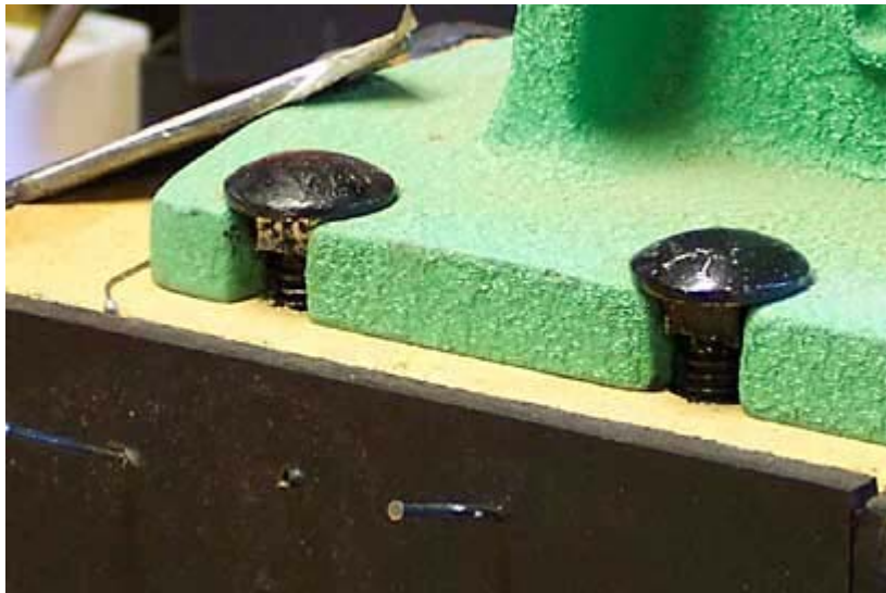
Carriage bolts fit into slotted press flanges.
