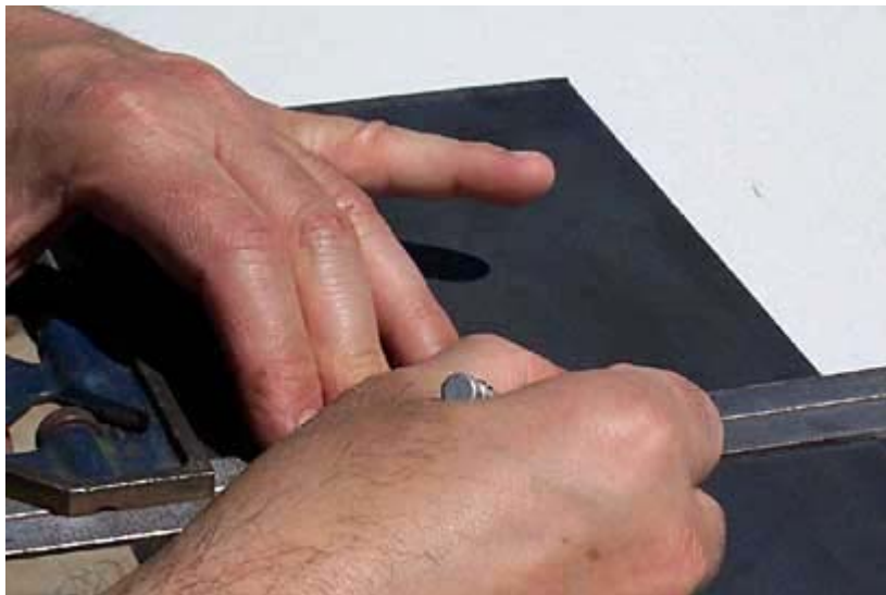
Scribing the centerline & vertical or Y-axis of the outboard hole.
