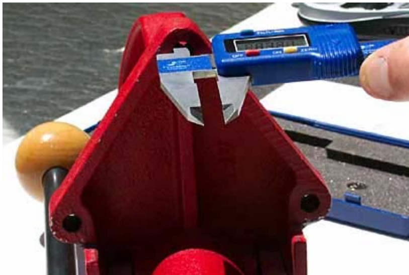
Measuring the width of the holes with the inside jaws.
