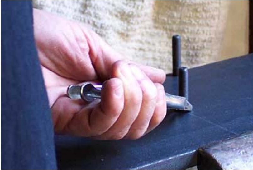
Turning studs in with locking pliers.
