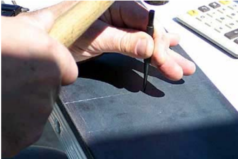
Center punching the steel plate.
