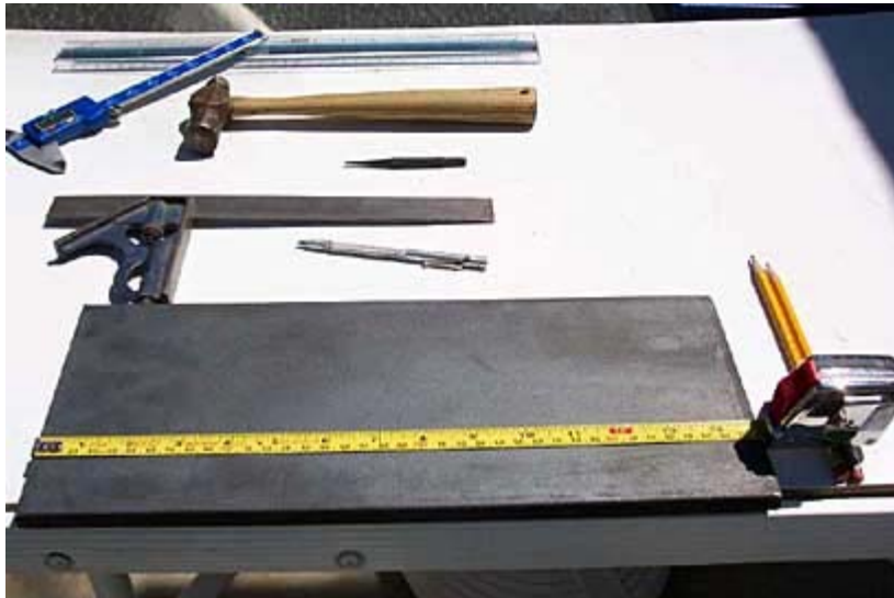
Measuring the centerline & vertical or Y-axis of the outboard hole.
