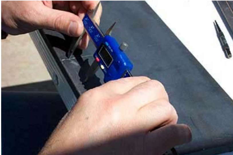
Marking the vertical or Y-axis center-to-center measurement of the right inboard hole.
