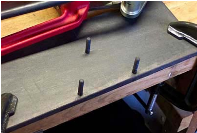
Finished plate C clamped to bench. Look carefully and you can see the scribed lines in the plate.
