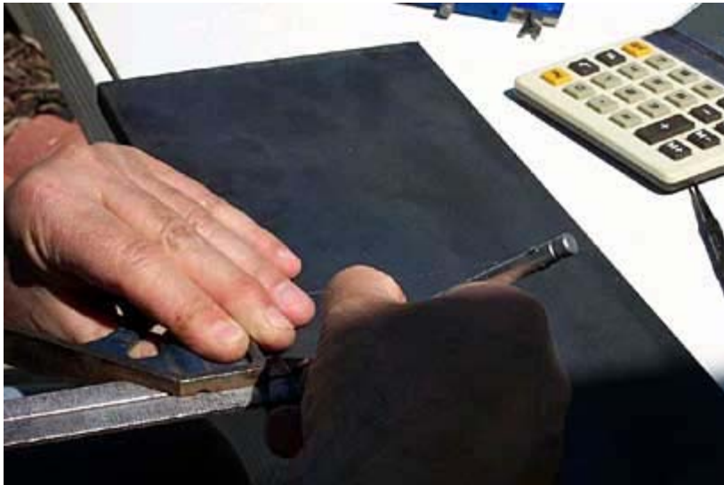
Scribing the line for the horizontal inboard holes.
