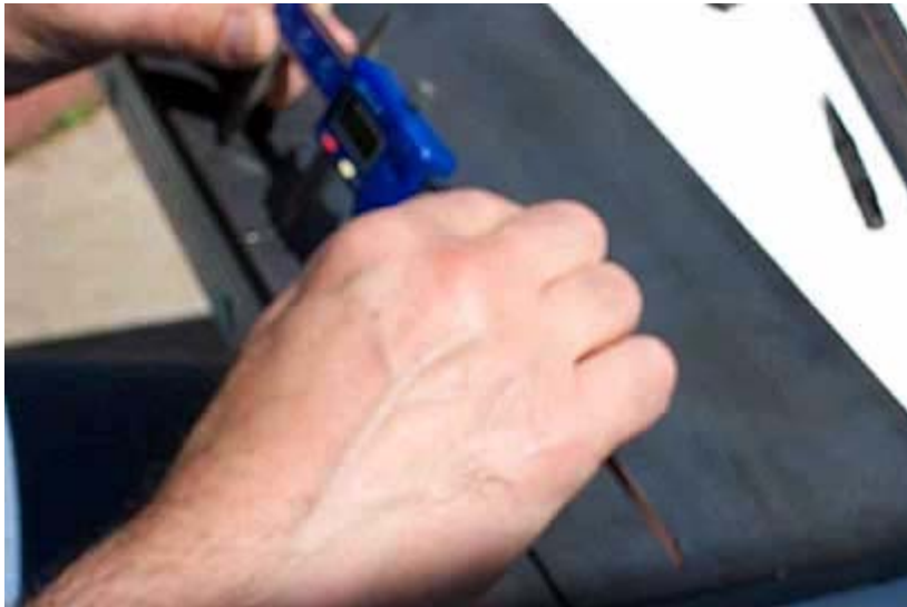
Marking the vertical or Y-axis center-to-center measurement of the left inboard hole.
