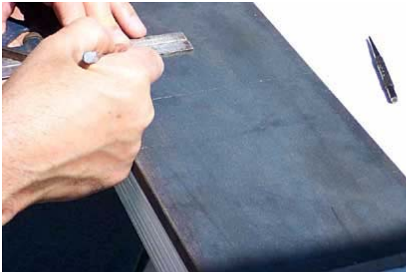
Scribing the line for the vertical or Y-axis center-to-center measurement of left inboard hole.
