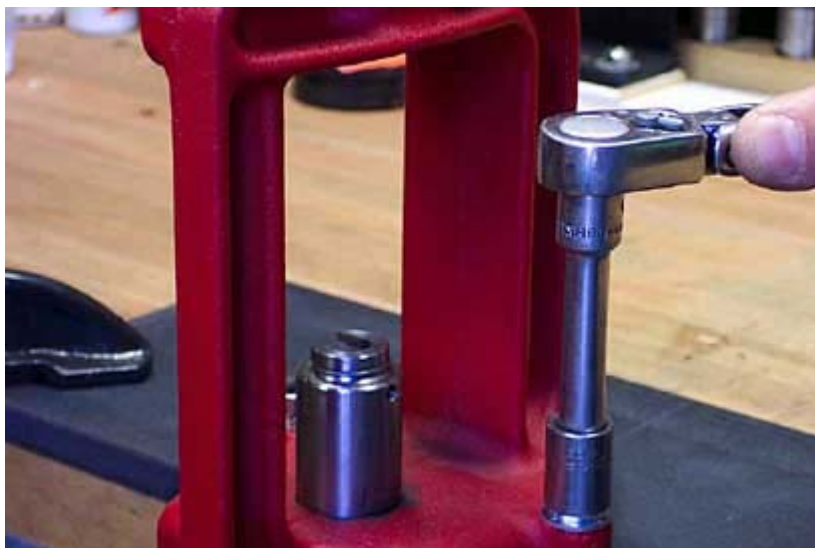
Tightening down the nuts.
