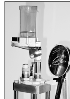
2 SIZE THE CASE Place a shell in the shell holder. Rotate the turret to position the full length sizer over the case. Firmly raise the ram to the top and stop.
