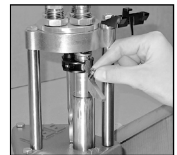
3 SELECT THE CORRECT LEVER PRIME ASSEMBLY (large or small). With clean fingers, place the correct size and type of primer in the primer guide. (This operation is greatly speeded by using the Lee Safety Prime primer feeder. Never touch the primer from box to shell.) Seat the primer by lowering the ram—lifting up on the press lever. Lift firmly enough to seat the primer flush to slightly below flush of the case head.
