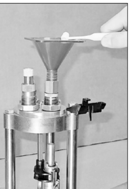
3 SELECT THE CORRECT LEVER PRIME ASSEMBLY (large or small). With clean fingers, place the correct size and type of primer in the primer guide. (This operation is greatly speeded by using the Lee Safety Prime primer feeder. Never touch the primer from box to shell.) Seat the primer by lowering the ram—lifting up on the press lever. Lift firmly enough to seat the primer flush to slightly below flush of the case head.
