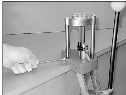
FIGURE 1 Attach the Classic Turret Press to the front edge of a sturdy bench using three 3/4 or 5/16 inch bolts.
