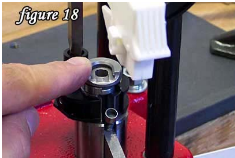
Notice the proximity of the shellholder, primer arm and primer feed The Safety Primer Feed is slid into the bracket, and the ram is raised to full height so the bracket can be adjusted at the proper angle.
