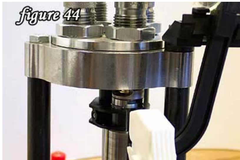
Raise ram, resize case and expel fired primer...
