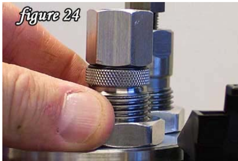
Screw the Lee expander die in until it touches the shellholder, and then back out one full turn.
