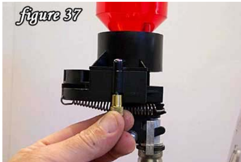
Installing brass hopper nuts
