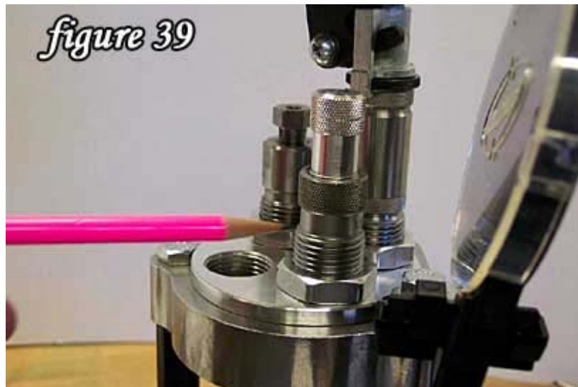
Lee bullet seater die installed
