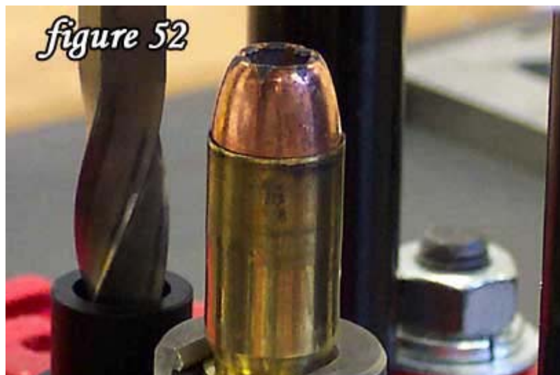
Round has been through the bullet seating die and the crimp and post size die. A
