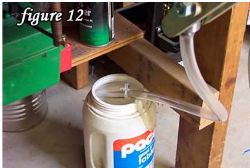
With cap removed, PVC Drain Tube is routed to waste container
