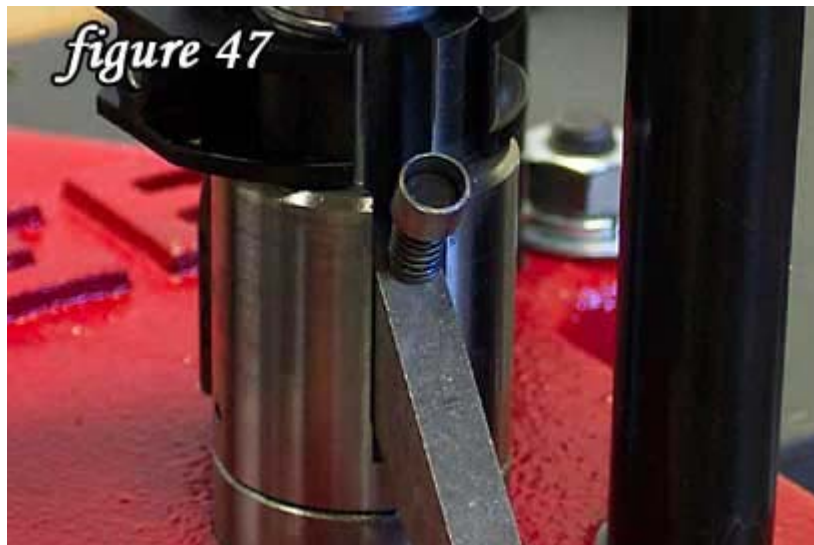
New primer is now seated and brass case is moving toward the expander and
